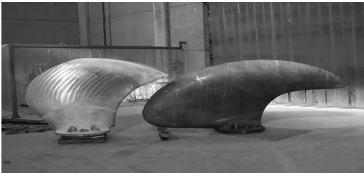
Figure 5. The striking difference between two equivalent propeller blades: CLT, left, and high skew conventional propeller blade, right, for a modern Ro-Pax.
