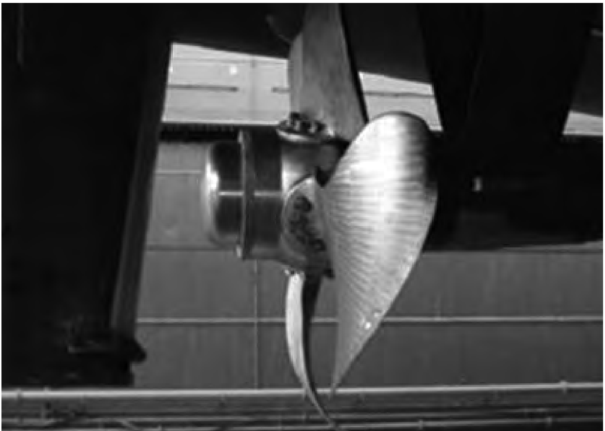
Figure 2 A CP Kappel propeller, note the propeller tip curled toward the suction side.
