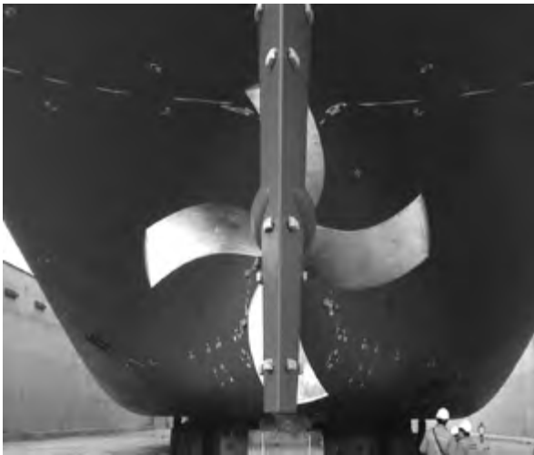
Figure 9. FP CLT propeller fitted on "JS Greenstone", 12,000 m 3 LEG carrier.
