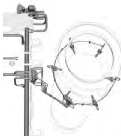
Fig. 7: Pulse lubricating system with pulse jet technology to distribute the oil evenly on the cylinder liner surface
