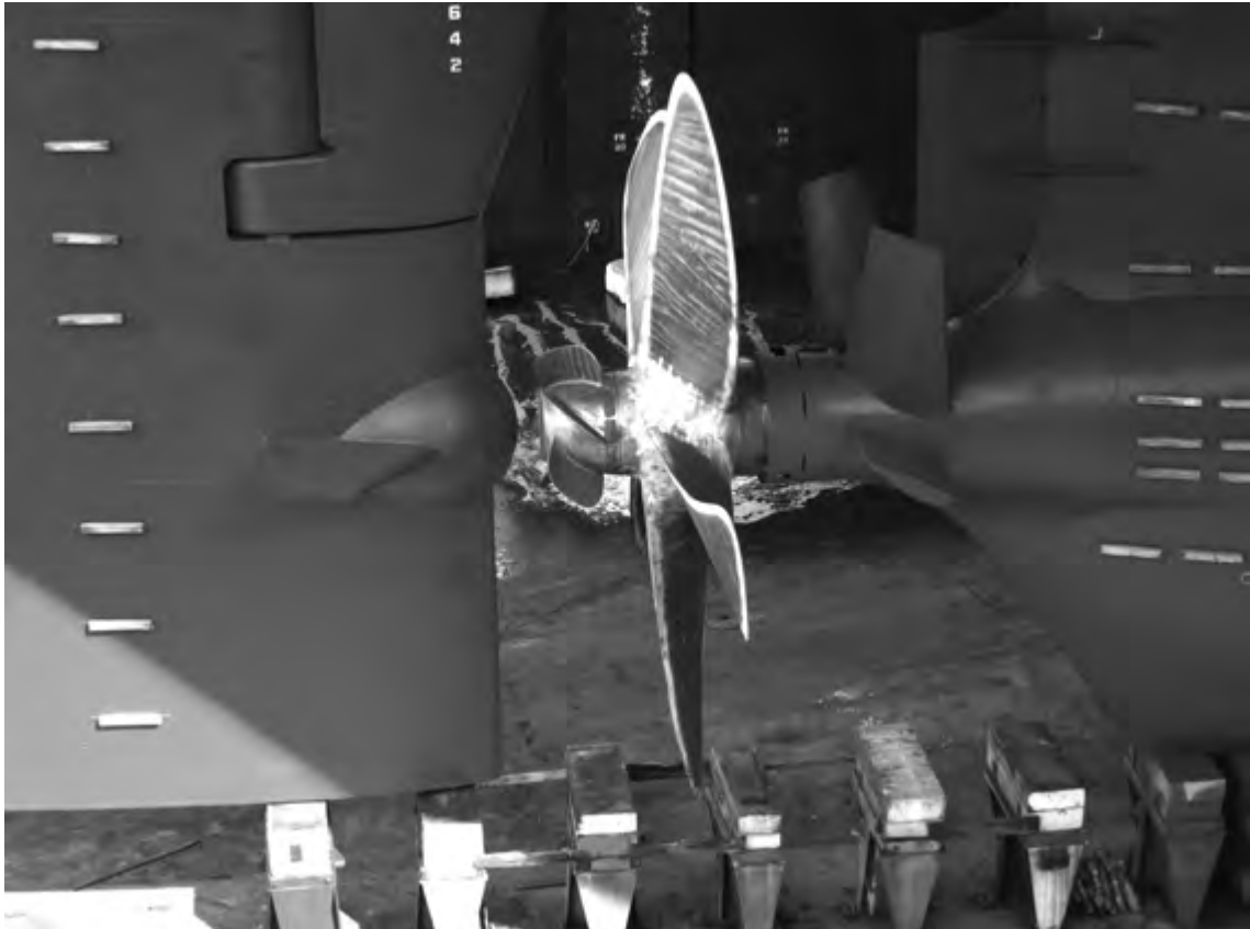
Figure 8. Superabundance of PIDs in a recent newbuilding, this is definitely a dont!
