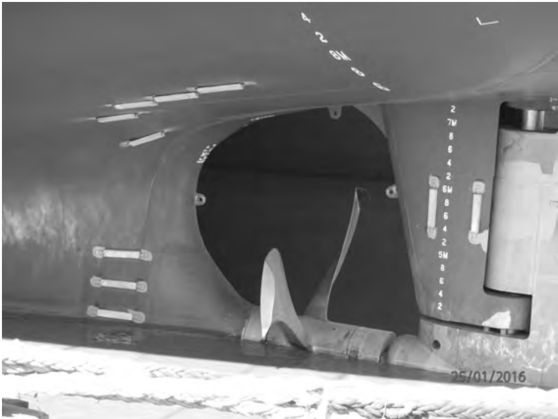
Figure 10. FP CLT propeller fitted on "Giancarlo D", 19.800 DWT chemical tanker
