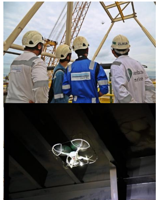
Figure 2: Collaborating with Classification Societies in the adoption of drones for remote inspections at height (top) and in confined spaces (bottom).
