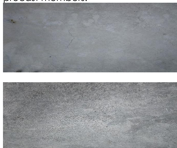
Figure 1: Drying shrinkage crack on normal Grade 40 MPa concrete with granite aggregates (Top), No Crack on Grade 40 MPa light weight concrete (Bottom)
