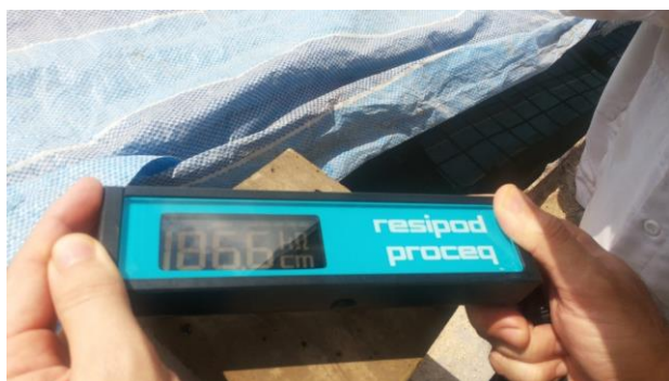
Figure 3: Wenner Probe reading to measure concrete mix durability
